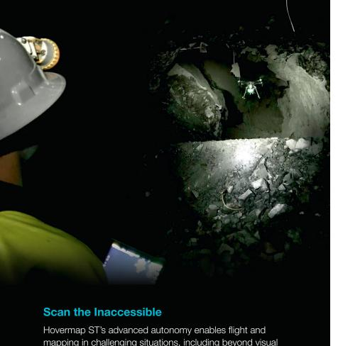
Hovermap ST's advanced autonomy enables flight and mapping in challenging situations, including beyond visual line of sight and communication range even in GPS-denied environments. Send a Hovermap ST enabled drone to explore and map previously inaccessible areas, providing new, valuable insights while the operator remains in a safe location.
